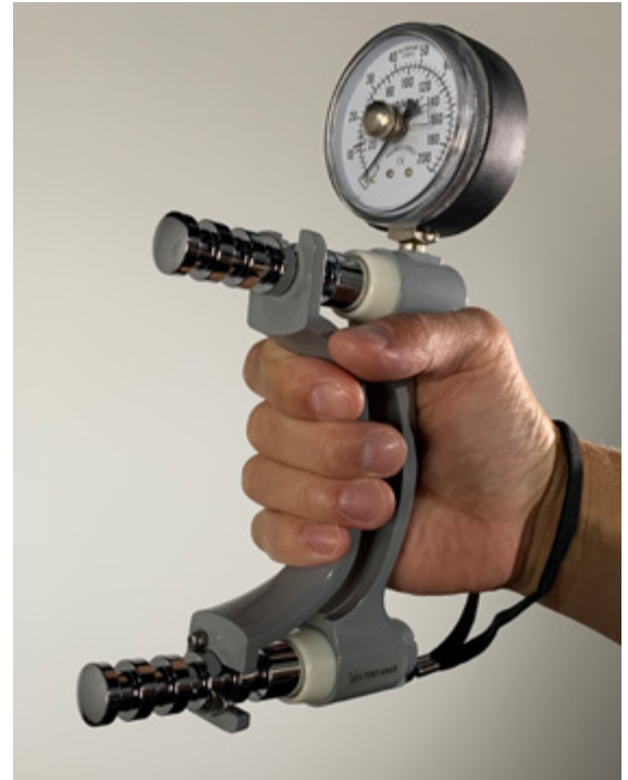
Figure 5-14. Hand Dynamometer. This instrument is commonly used by occupational therapists for hand rehabilitation. The dial displays pounds of force generated by the grip.
